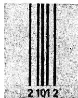
Fig. 5. From photographic exposures of the central line (0) and two double lines (1,1 and 2,2) on an Ilford H.P.S. Plate. Line 0: exposure time 7.5 sec., Q_0 = 0 . Lines 1,1: 15 sec., Q_0 = 0.00657 watt/cm. Lines 2,2: 15 sec., Q_0 = 0.0183 watt/cm. Voltage of accumulator: 0, 6 and 10, respectively. Substance: colourless liquid paraffin. Light source: straight wire lamp without filter.
